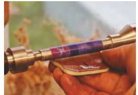
▲ Pic.10 Moving onto MicroMesh pads, keeping them wet allows you to achieve the ultimate mirror-like finish
